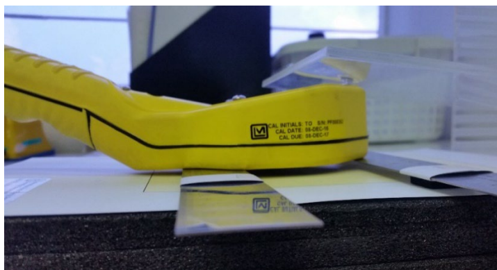
Fig.1. The large detector can be measured the whole area of contaminated surface in one time
