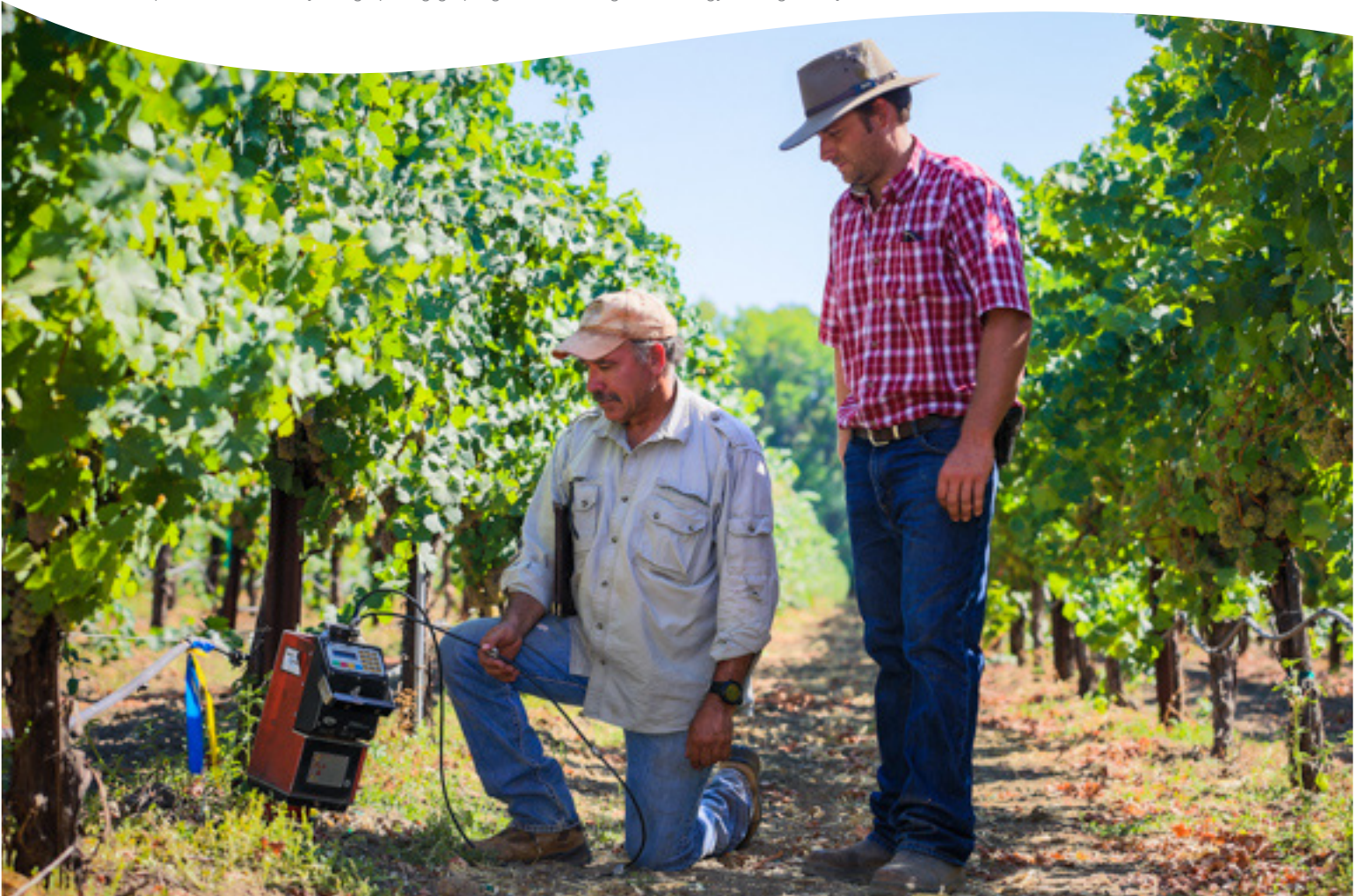
ภาพ A neutron probe to take soil moisture measurements at Rooster Vineyard in Kelseyville. ที่มา: http://www.lakecountywinegrape.org/grape-growers-leverage-technology-manage-vineyard-water-use/
